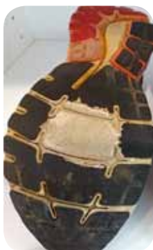
Fig. 4: Excessive outsole wear in central ball of foot region
