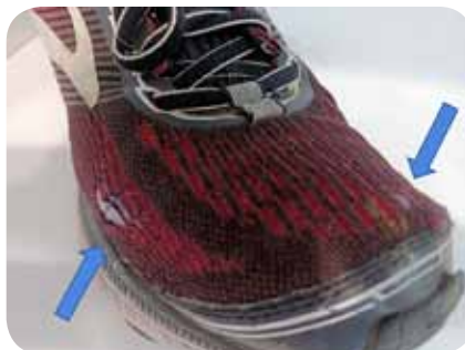
Fig. 8: Tearing of upper in toe area over big toe and little toe due to shoe too snug in these areas
