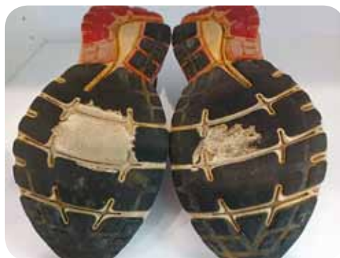
Fig. 5: Asymmetric wear between right and left shoe
