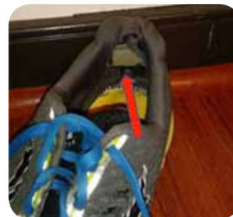
Fig. 9: Interior of heel counter worn through by heel friction
