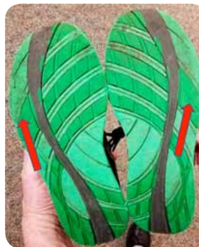
Fig. 2b: Wear on lateral side of outsole under forefoot but not heel, typical of runner who is a forefoot striker
